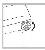
2. If the floor is uneven, the front feet of the machine may be adjusted until it reaches a horizontal position (the angle of inclination must not exceed 2 degrees). If the appliance is levelled correctly, it will be more stable and much less likely to cause vibrations and noise while it is operating, particularly during the spin cycle.If it is placed on carpet or a rug, adjust the feet in such a way as to allow a sufficient ventilation space underneath the washing machine.
